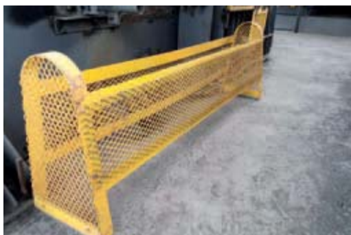
Mechanic guarding rectification
